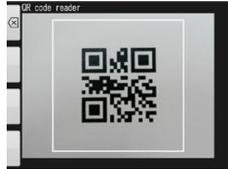
When scanned successfully, the message shown on the right will appear on the screen. Press "OK" to store the information.
