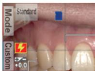
When the flash mode icon
